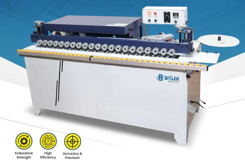
High-speed Edge Banding Machine BEB-160 not only increase productivity and cost efficiency in the woodworking industry, but also offer better quality, flexibility in use, full automation, time savings and easy integration with other machines. Moreover, additional features such as high-power spindle and motor, glue removal system, silent polishing motor, and adjustable pressure settings, as well as stable and smooth double-row pressure rollers.
