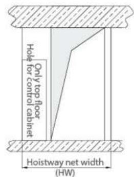
Reserved Hole Drawing For Enter And Exit At Top Floor
