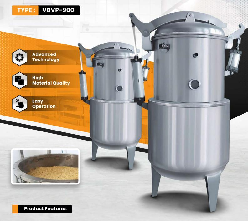
The vacuum pot is heated by steam, wherein sugar syrup is infiltrated into beans within short time under vacuum pressure. The processing of infiltration is done in sealed space without oxidation, which reduces loss of nutrition and maintains original color and appearance with good taste.
