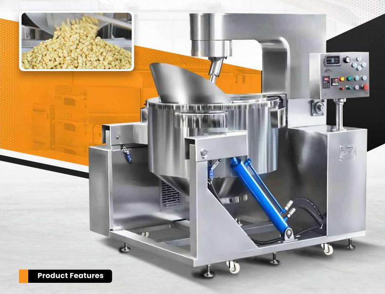
Vergon brand big capacity popcorn machine is researched and developed from the traditional popcorn machine by providing mixing and coating system and improving heating source. It can reach high temperature rapidly to make sure popcom are produced with perfect mushroom shape. The popcorn machine can be heated by LPG gas and electric induction.
