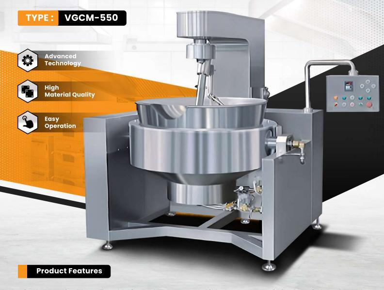
It is characterized by adjustable fame that can reach high temperature within short time and enable materials with pleasant taste and smell. Its planetary stirring devices ensure thorough mixing efficiently while decreasing production cost for customers. It is widely used for its compact size, easy maintenance and satisfactory performance.
