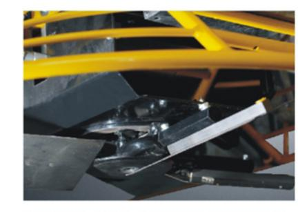
Super heavy-duty gearbox and spider assembly stands up to the most grueling job.
