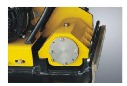
Cast Iron wear resistant lubricated vibrator assembly.
