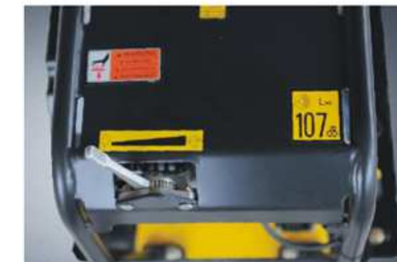
Sturdy protected throttle lever.
