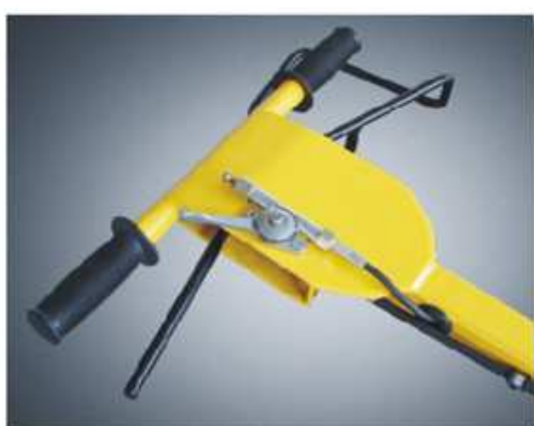
Deadman control and reversing protection.
