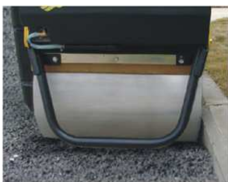
Narrow overhang for operation close to walls and curbs.
