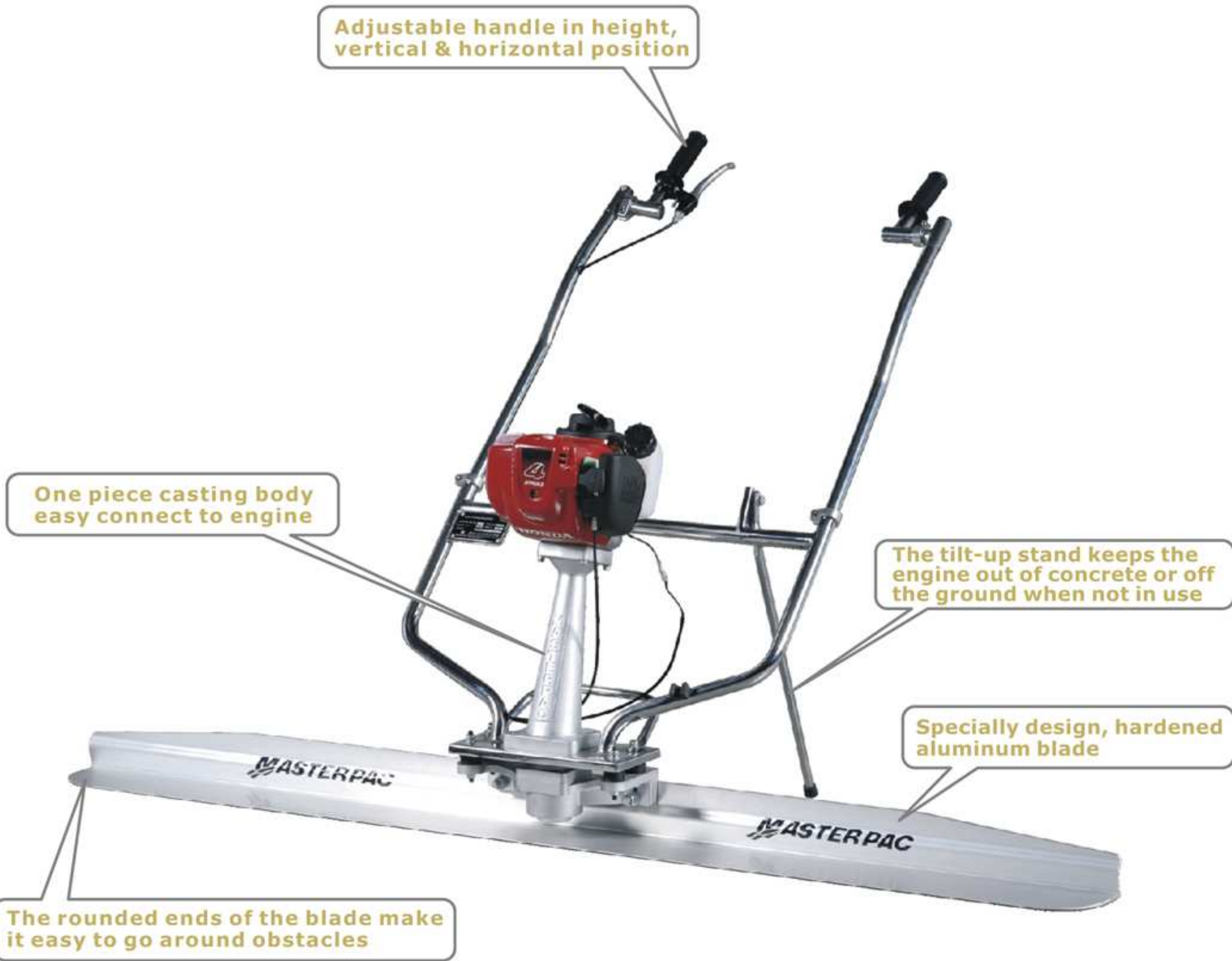
The blade is easily changed within 2 minutes, Masterpac blades are available in length from 4ft. (1.2m) to 16ft. (4.9m).
