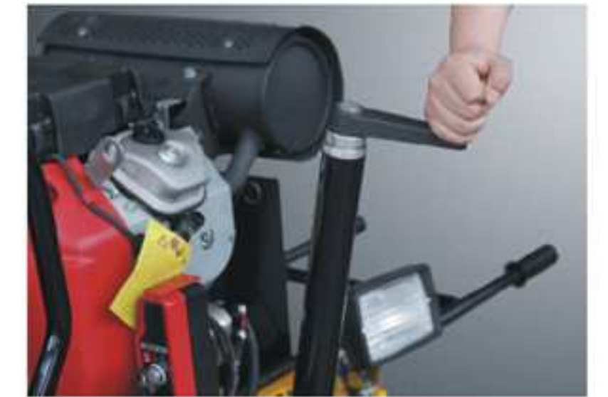
Fine hand control for blade pitch ensures precise blade adjustment.
