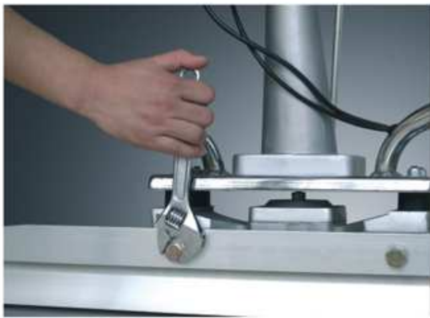
The blade is easily changed within 2 minutes, Masterpac blades are available in length from 4ft. (1.2m) to 16ft. (4.9m).
