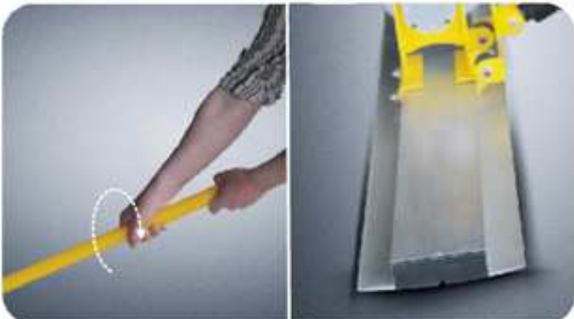
Turning the handle to the left, to make the blade incline backward, pulling and spreading the concrete.
