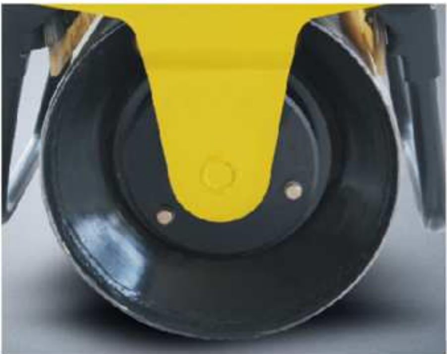
Thick drum shells for longer drum life.
