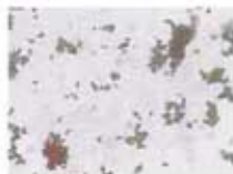
Water samples from well treated water tank inner wall of water compressor show rust particle under electron microscope.
