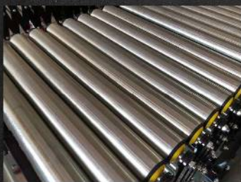
50mm Galvanized Steel Rollers
