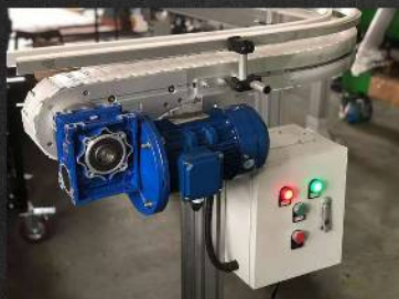
Control Box Power On, Start, Help, Stop
