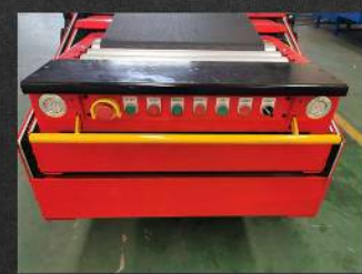
Load, Unload, Up, Down, Emergency Stop, Light OFF/ON buttons
