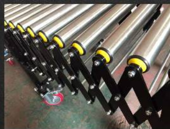
5mm Reinforced Steel Side Links
