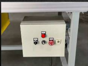
Control Box Forward, Stop, Reverse, Emergency Stop Speed Knob
