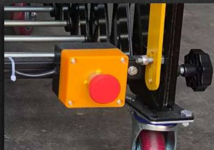
E-Stop Button at rear for emergency stop button
